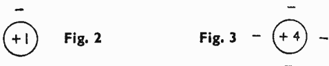
Fig. 2. For some purposes the atom diagrams can be greatly simplified by lumping the filled shells in with the nucleus and showing only the net electric charge inside a circle. Each of the electrons left over—the valency electrons—is represented by a minus sign. The diagram here replaces the sodium diagram in Fig. 1 and also a number of even more complicated ones.
